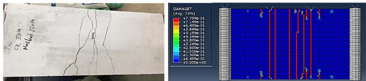
Comparisons of slab S4 failure mechanisms using numerical and experimental methods
