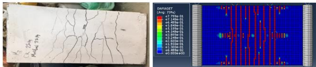
Comparisons of slab S3 failure mechanisms using numerical and experimental methods
