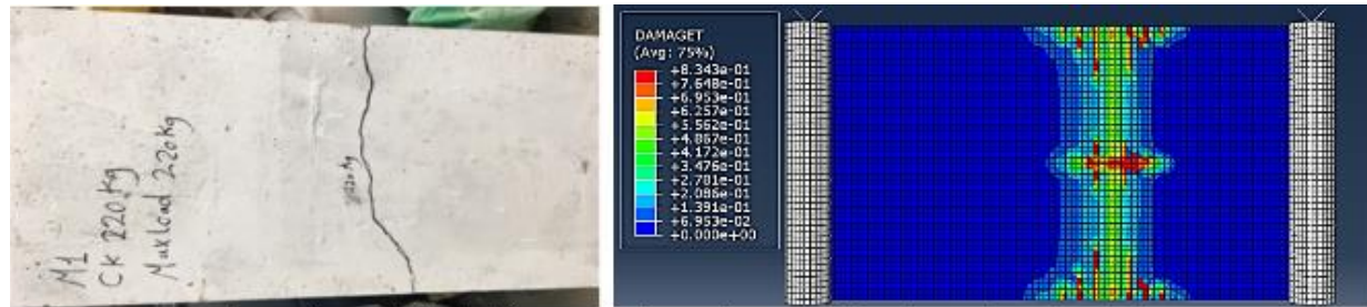
Comparisons of slab S1 failure mechanisms using numerical and experimental methods
